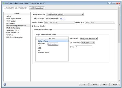
Use the build option to specify how the build process should take place during code generation.
