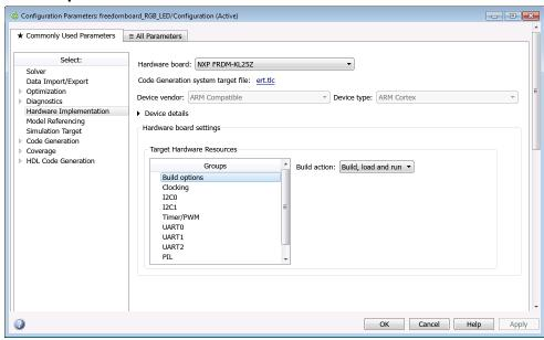
To specify how the build process takes place during code generation, select build options.
