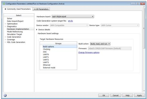
To specify how the build process takes place during code generation, select build options.
