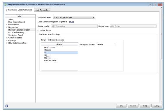
Use the PIL options to set PIL (Processor-in-the-Loop) communications parameters.
