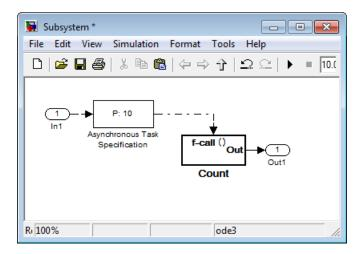
If the **Task priority** parameter is set to 10, the Async Interrupt block in the parent model must also have a priority of 10. If the parameter is set to [], the priority of the Async Interrupt block can be a value other than 10.
